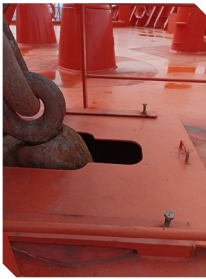
Sealed anchor chain hawse pipe hole [Courtesy of ReCAAP Focal Point (Philippines)]
