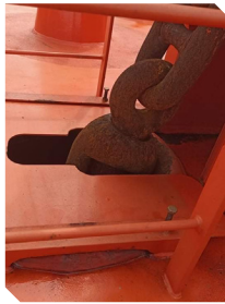
Sealed anchor chain hawse pipe hole [Courtesy of ReCAAP Focal Point (Philippines)]
